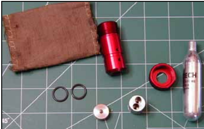
Photo 1: The individual components of the 12-gram CD3 are shown. The red anodized barrel shows two holes: the lower is the vent port for the CO 2 the upper is the vent for pyrogen gases. The Nomex shield is used to attenuate the pyrogen gases. The e-match holder clearly shows the wells for holding redundant e-matches. The grid in the background is of one-inch squares.
