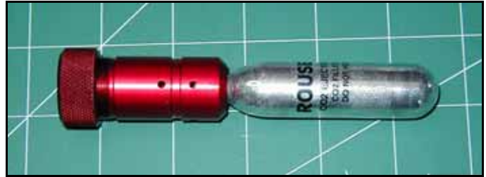
Photo 2: This shows the assembled mechanism without the Nomex shield and without the e-match electrical harness. The e-match harness would exit through the hole in the back of the knurled knob on the left. That whole end of the mechanism would be covered by the Nomex shield.
