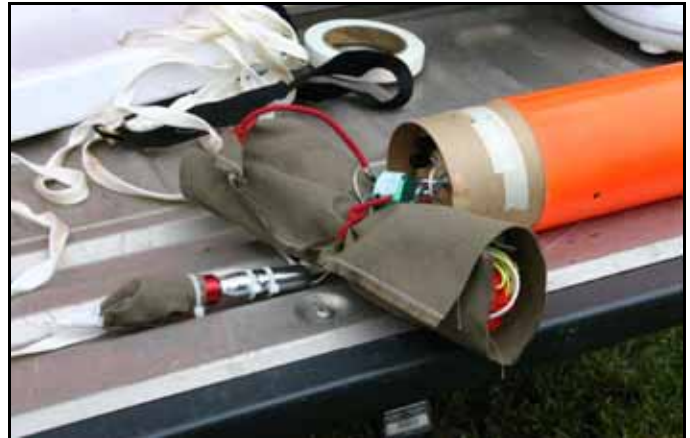
Photo 3: The tie-wraps used to attach the CD3 to the nylon recovery harness are clearly shown in this photo. The placement of the Nomex shield is also shown. The left (aft) end of the Nomex shield is closed with masking tape. The e-match electrical harness exits from that end and is routed along the recovery harness to the altimeter connectors on the aft end of the payload bay. The large Nomex shield in between the CD3 assembly and the aft end of the payload bay is the main parachute reefed with a Defy Gravity Tether. Photo courtesy of Corrie Wolfe.
